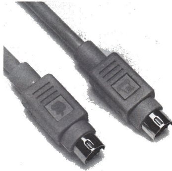
Figure 3-2. The 8-Pin, Mini-Circular Connector
